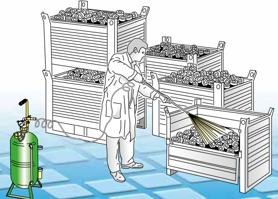
Spraying antioxidant, oil, diesel oil on mechanical parts
